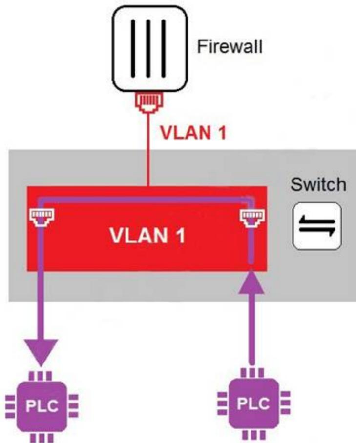
In the topology shown in the exhibit, both PLCs can communicate directly with each other, without going through the firewall. Which statement about the topology is true?
