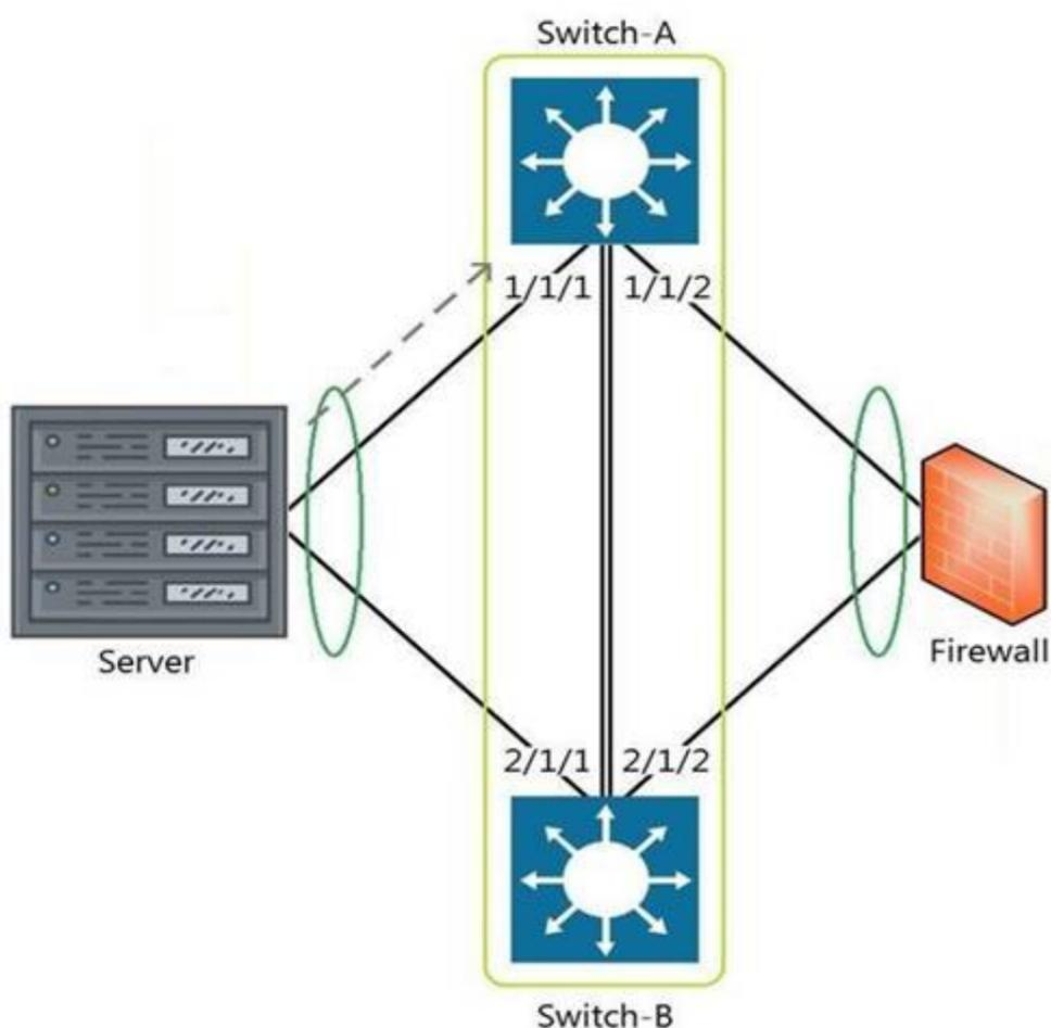
The above scenario shows a packet from the Server destined for the Firewall. Switch-A and Switch-B are bundled as VSF stack. The LAG between the VSF stack and the firewall indicates a hash function to forward the packet on port 2/1/2.
