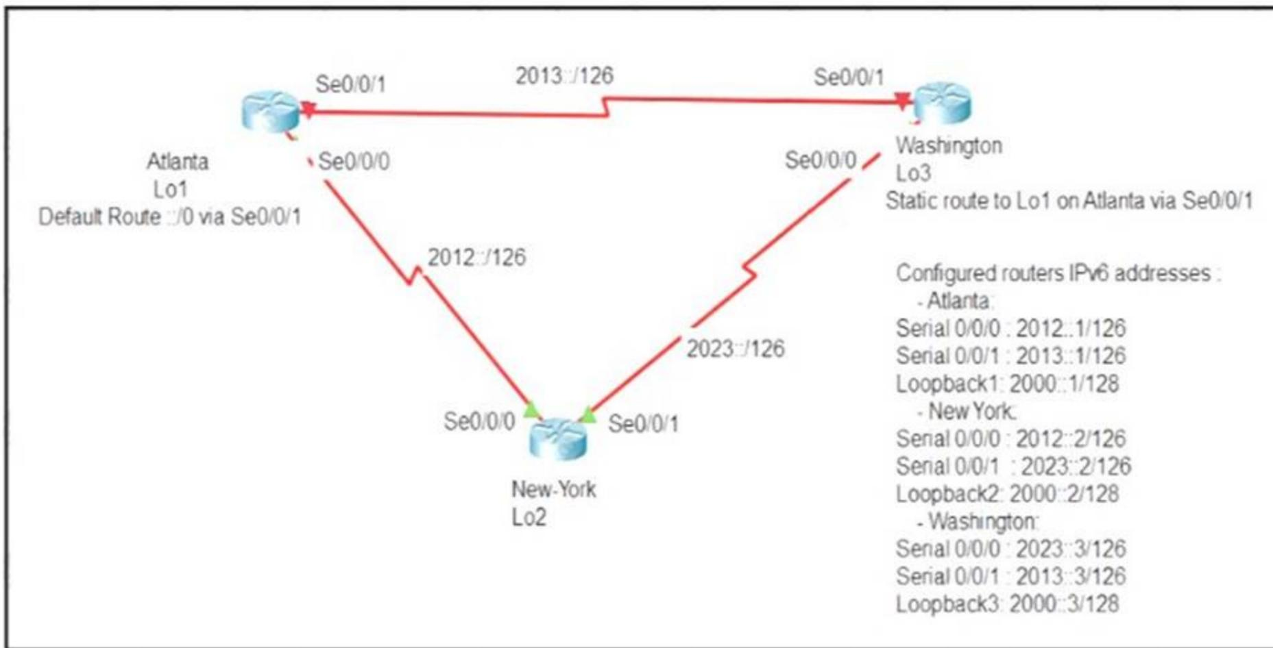
An engineer is configuring the NEW York router to reach the Lo1 interface of the Atlanta router using interface Se0/0/0 as the primary path. Which two commands must be configured on the New York router so that it can reach the Lo1 interface of the Atlanta router via Washington when the link between New York and Atlanta goes down? (Choose two)
