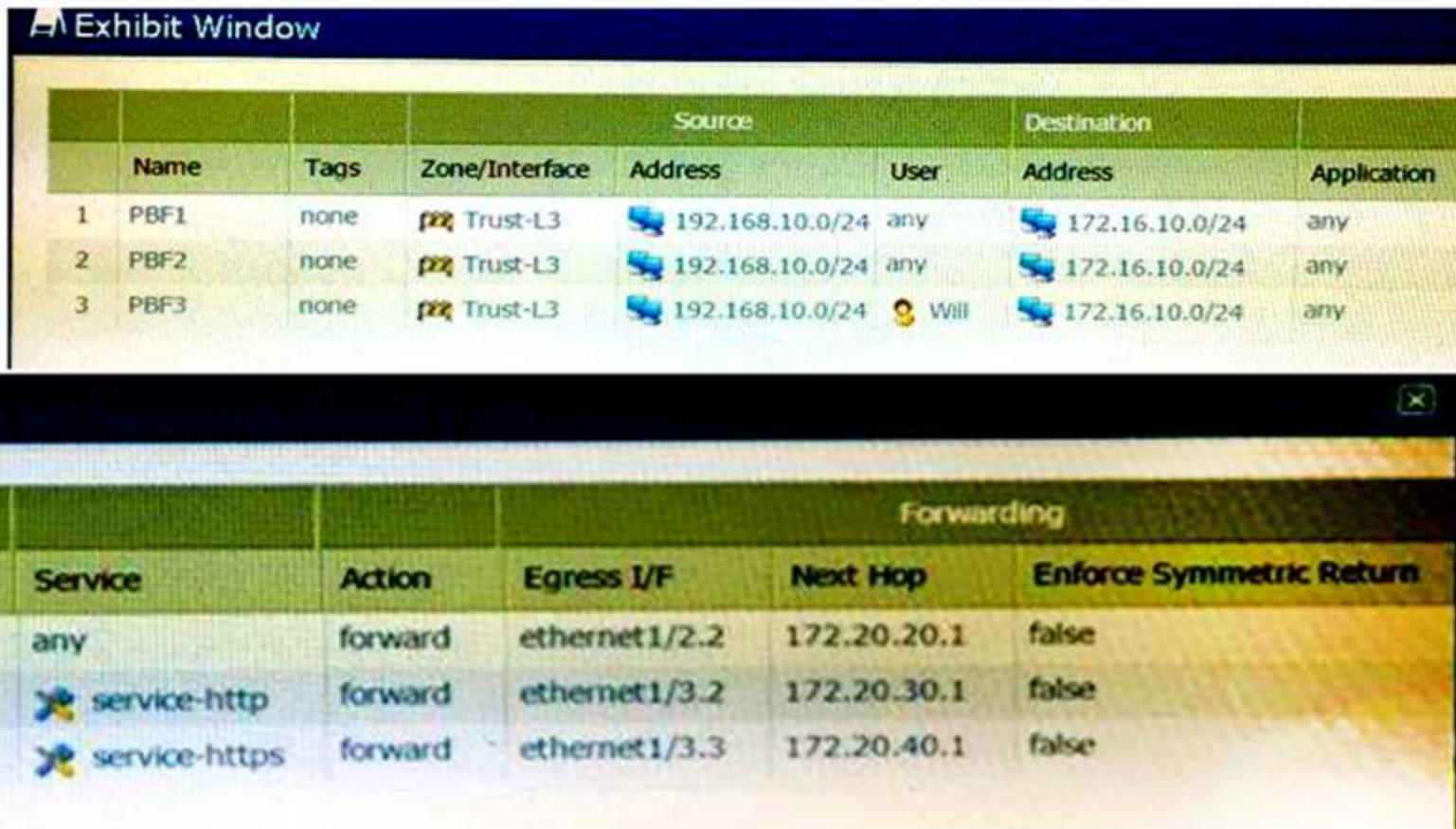
The screenshot shows two configuration windows from a Palo Alto Networks firewall. The top window is titled 'Exhibit Window' and displays a table of Policy-Based Forwarding (PBF) rules. The bottom window displays a 'Forwarding' table.
