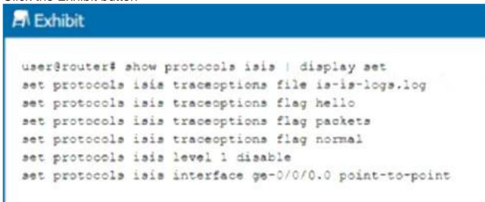
You are capturing logs to troubleshoot an issue with IS-IS; however, the logs are increasing in size too quickly. Referring to the exhibit, which configuration statement would solve this problem?
