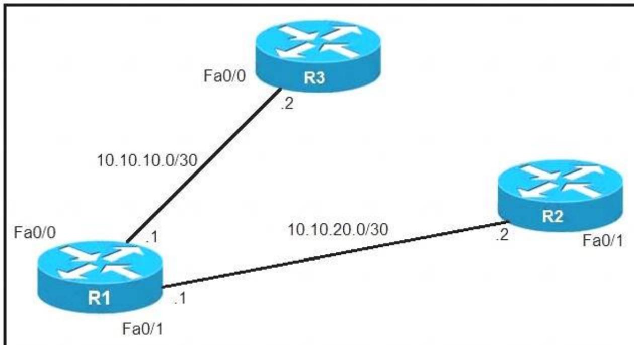
An IP SLA was configured on router R1 that allows the default route to be modified in the event that Fa0/0 loses reachability with the router R3 Fa0/0 interface. The route has changed to flow through router R2. Which debug command is used to troubleshoot this issue?
