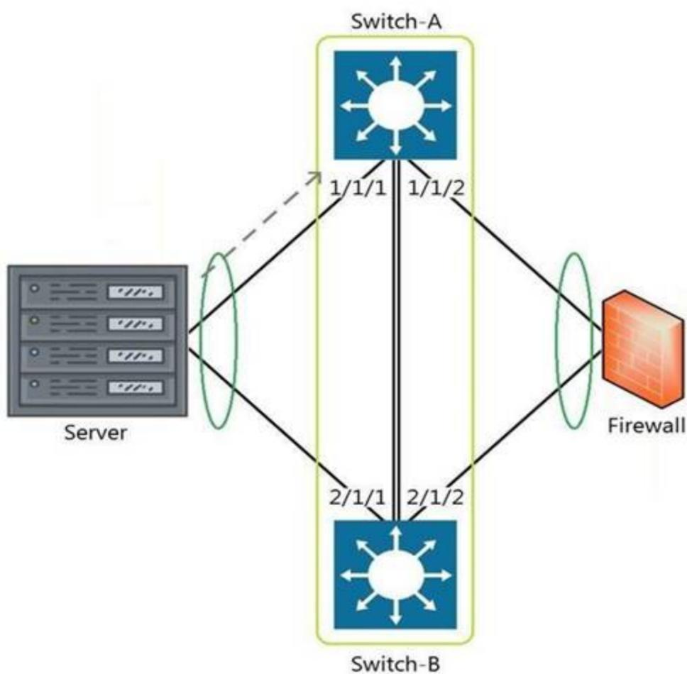
The above scenario shows a packet from the Server destined for the Firewall. Switch-A and Switch-B are bundled as VSF stack. The LAG between the VSF stack and the firewall indicates a hash function to forward the packet on port 2/1/2. Which statement is true regarding how Switch-A will forward the packet?
