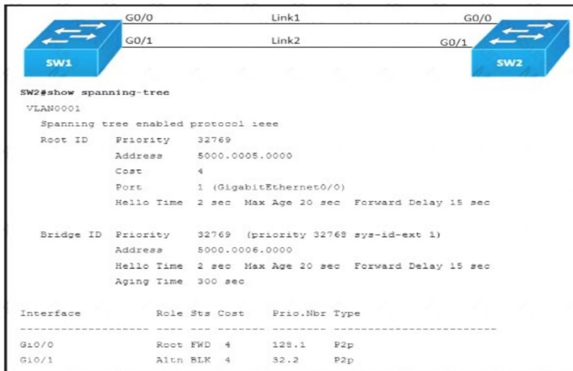
Link1 is a copper connection and Link2 is a fiber connection. The fiber port must be the primary port for all forwarding. The output of the show spanning-tree command on SW2 shows that the fiber port is blocked by spanning tree. An engineer enters the spanning-tree port-priority 32 command on G0/1 on SW2, but the port remains blocked. Which command should be entered on the ports that are connected to Link2 to resolve the issue?
