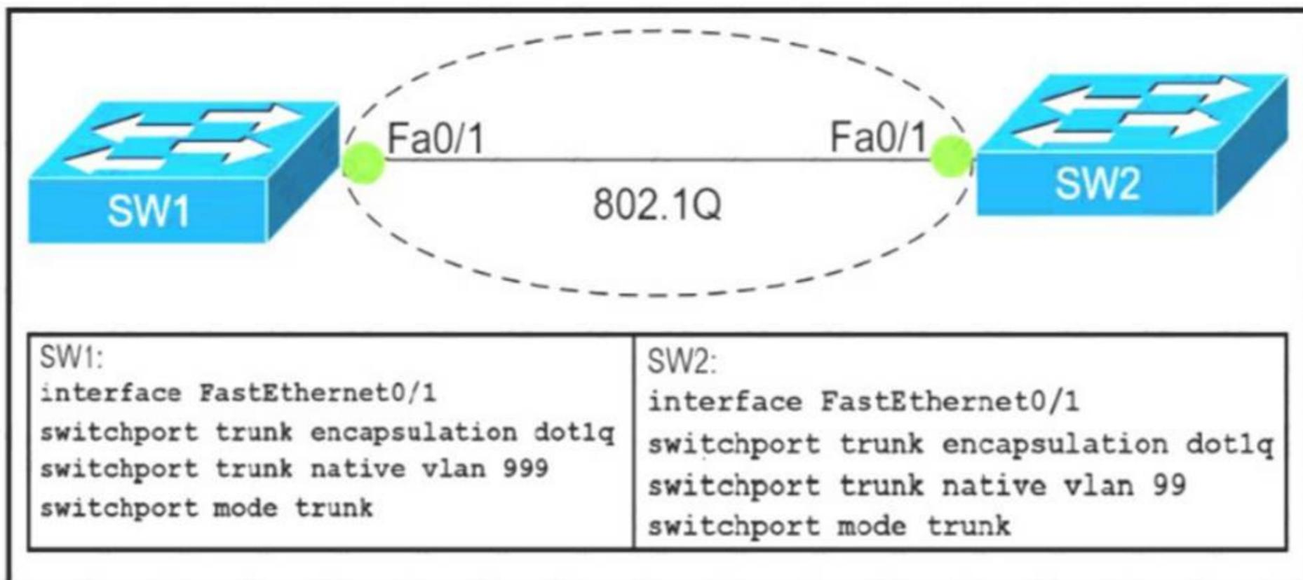
Which action do the switches take on the trunk link?
