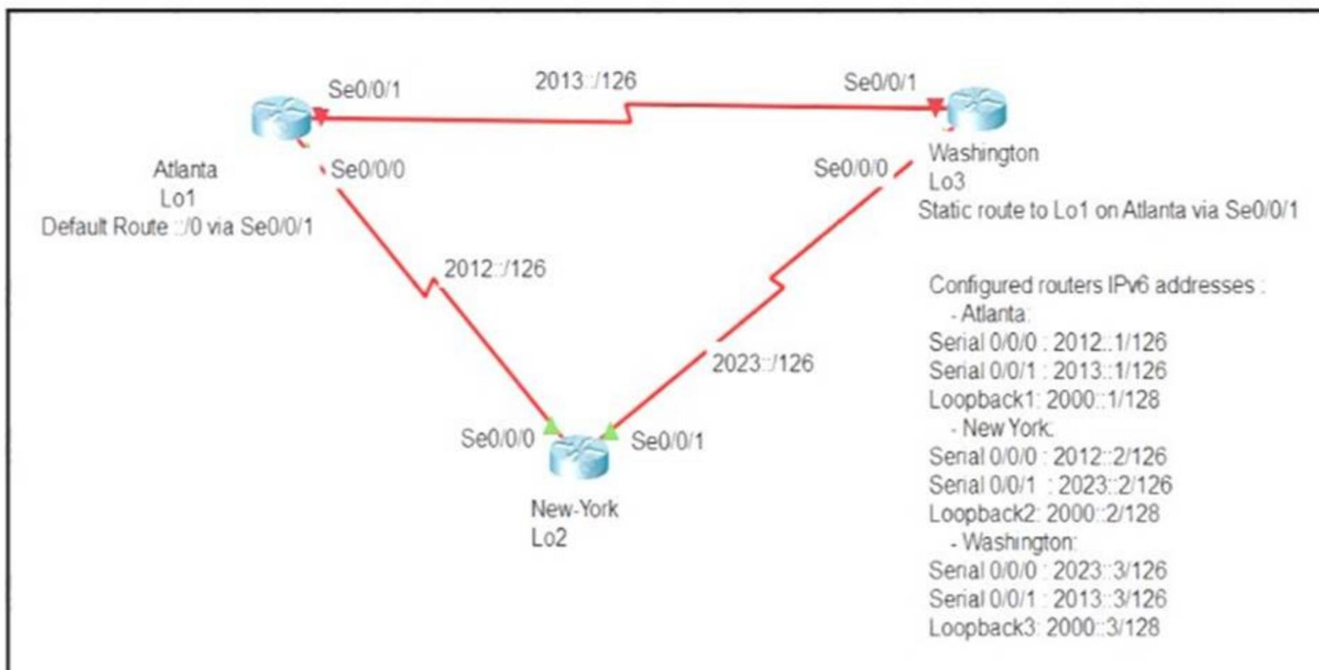
An engineer is configuring the NEW York router to reach the Lo1 interface of the Atlanta router using interface Se0/0/0 as the primary path. Which two commands must be configured on the New York router so that it can reach the Lo1 interface of the Atlanta router via Washington when the link between New York and Atlanta goes down? (Choose two)
