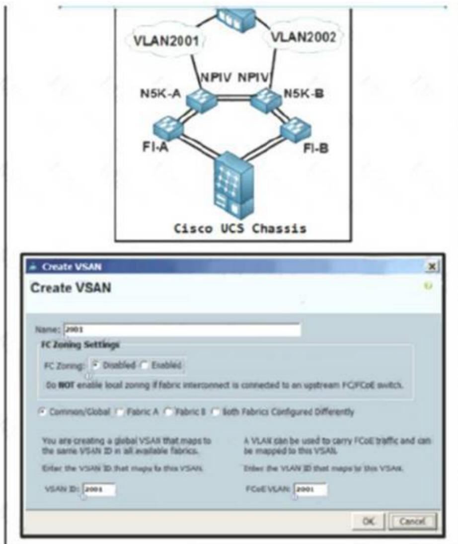
An engineer is configuring a VSAN on the network Which option must be selected to create the VSAN?
