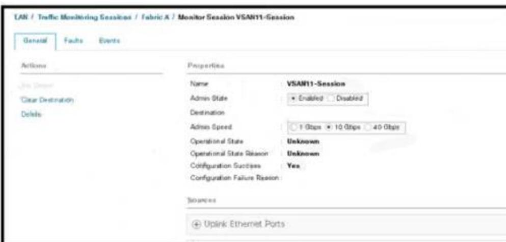
An engineer is creating a SPAN session to send a copy of all the Fabric-A VSAN 11 traffic on NSK\_1 to the monitoring laptop. The configurator that is presented has already been applied to Cisco UCS Manager. Which action completes the configuration?
