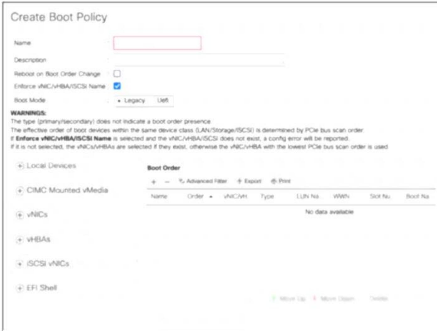
An engineer installs a new Cisco UCS B-Series server. The requirement is to install an operating system on a LUN that is provided by the Fibre Channel storage array. Which two steps must be configured in the boot policy to accomplish this goal? (Choose two.)
