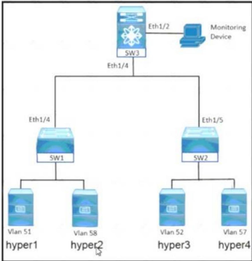
An engineer must monitor the Ethernet port and the corresponding VLAN traffic for the hyper4 device. The SW3 device is a Cisco Nexus 7000 Series Switch. Drag and drop the code snippets from the right into the boxes in the configuration to meet these requirements.
