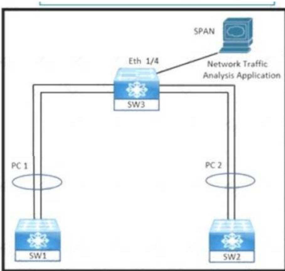
An engineer must monitor ingress traffic from SW1 and SW2 port-channel interfaces from SW3. Which configuration must be implemented to accomplish this goal?
