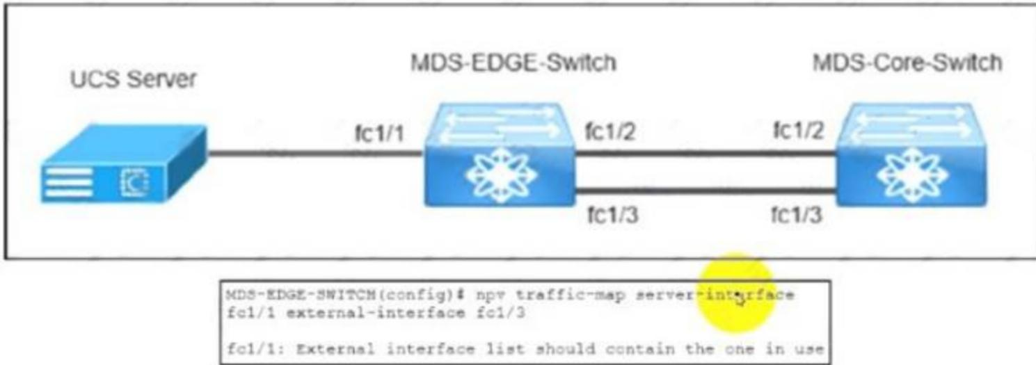
The MDS-EDGE-Switch and MDS-Core-Switch are configured with NPV and NPIV features. The FLOGI from Cisco UCS is received by the MDS-Core-Switch on interface fc1/2. An engineer tried to move all traffic between the MDS-EDGE-Switch and MDS-Core-Switch from interface fc 1/2 to fc1/3, but the attempt failed. Which set of actions completes the configuration?
