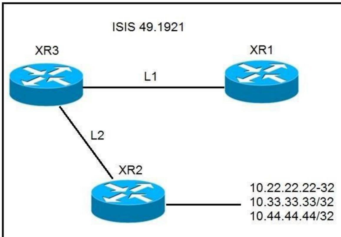
Refer to the exhibit. A network operator must stop 10.33.33.33/32 from being redistributed into Level 1 router XR1. Which configuration meets this need?
