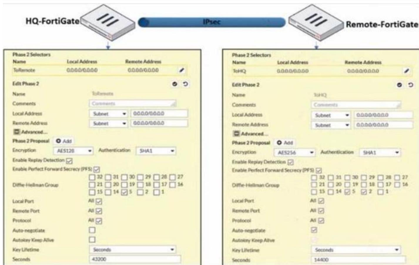
A network administrator is troubleshooting an IPsec tunnel between two FortiGate devices. The administrator has determined that phase 1 status is up, but phase 2 fails to come up.
