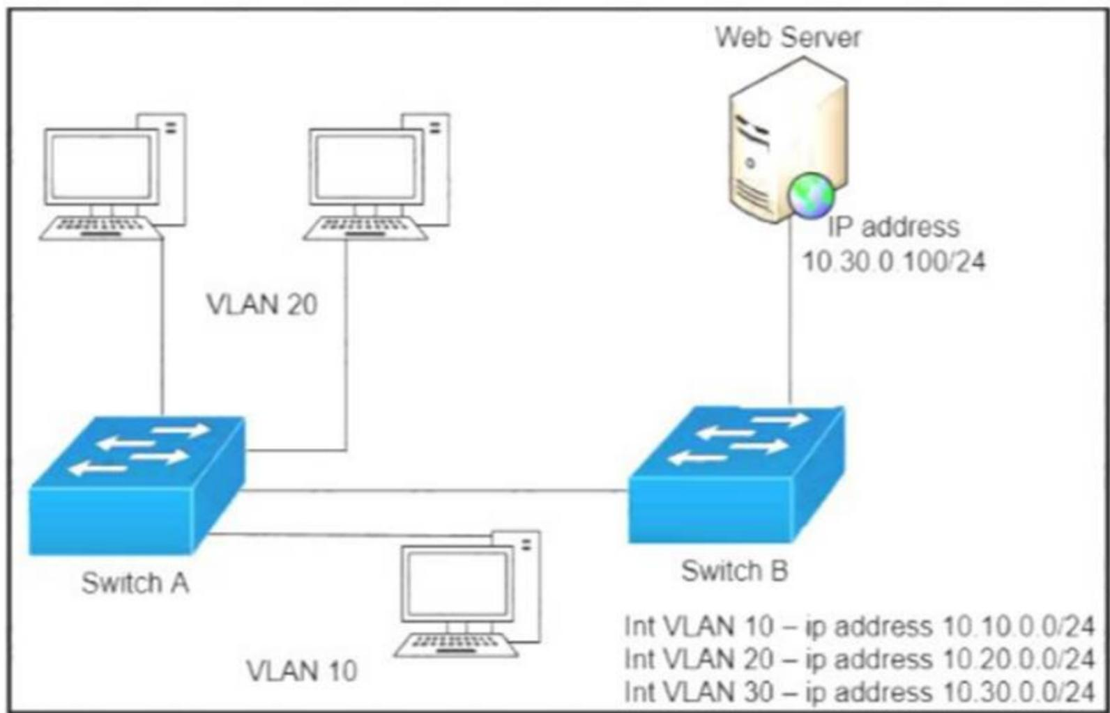
A network engineer must block access for all computers on VLAN 20 to the web server via HTTP All other computers must be able to access the web server
