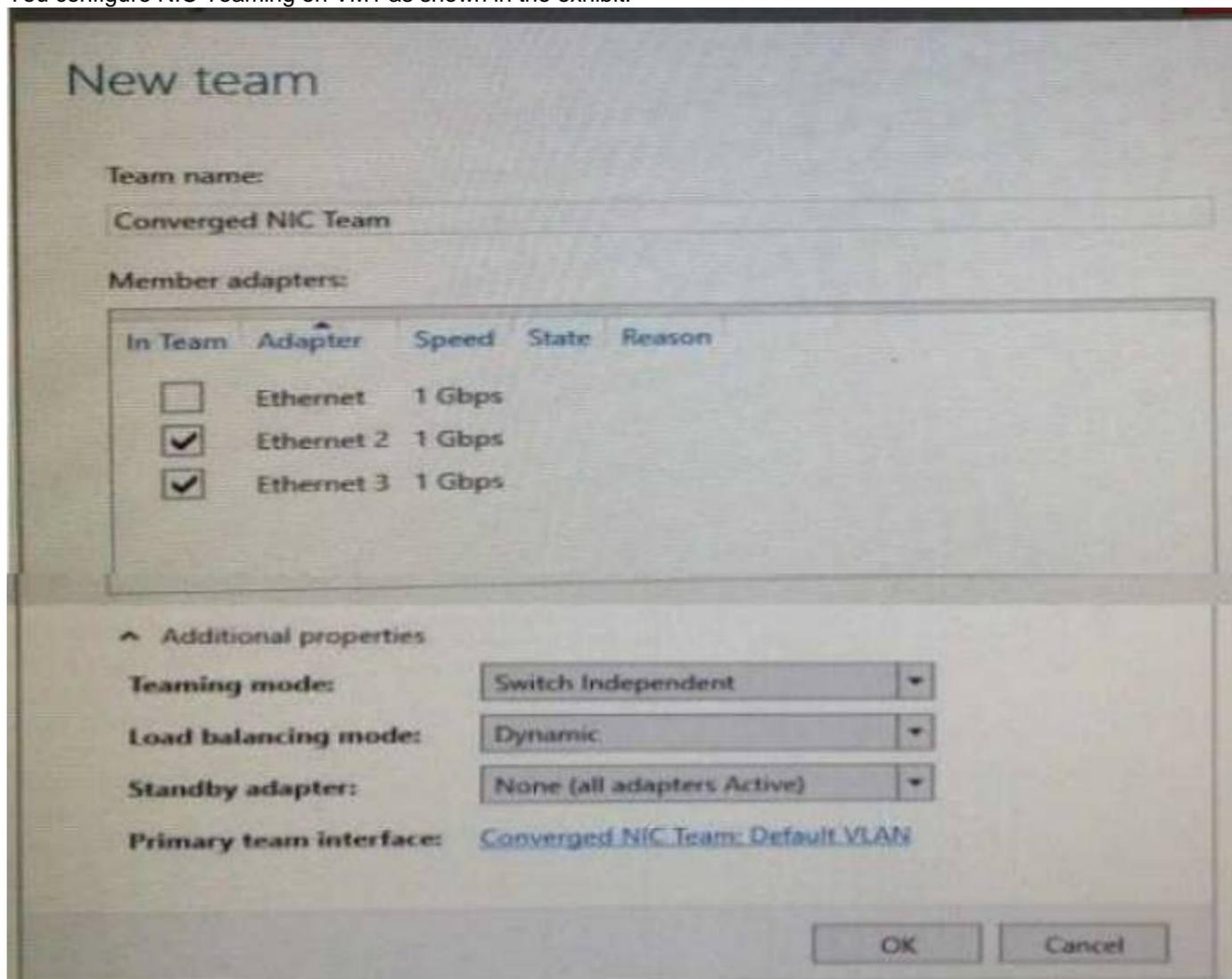
You need to ensure that VM1 will retain access to the network if a physical adapter card fails on Server1. What should you do?
