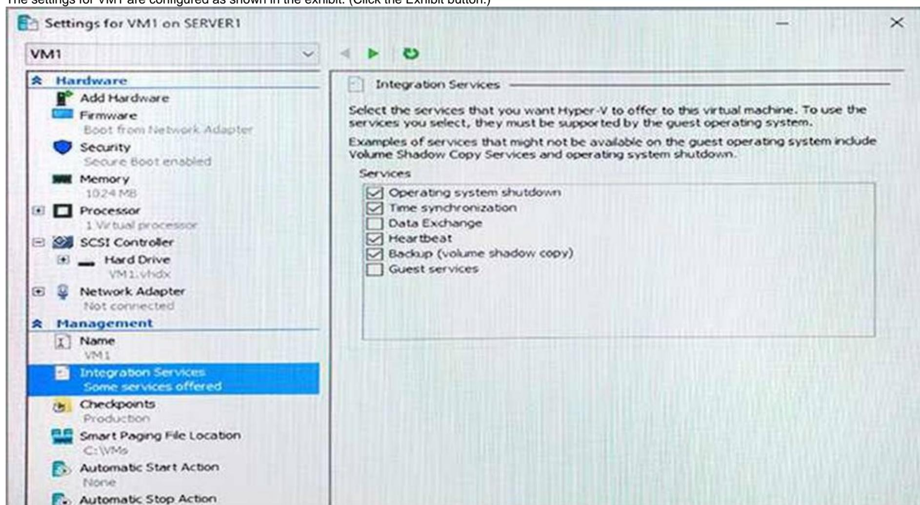
You need to ensure that you can use the Copy-VMFile cmdlet on Server1 to copy files from VM1. Solution: You enable the Data Exchange integration service for VM1.
